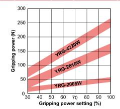
Graph shows a general guide to gripping power versus gripping power setting (%). Variations will appear in the actual gripping power.
